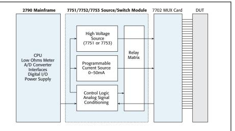
Multichannel resistance measurements for airbag inflator, harness, and connector testing
